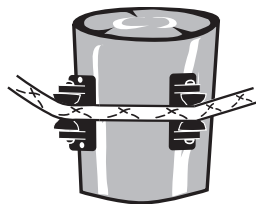
Use two ElectroBraid™ Roller Insulators around the back of the post to prevent the Braid™ from touching the wood.
